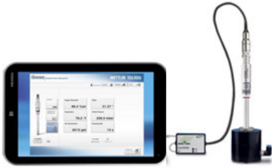
iSense software, iLink, and the InPro6860i (measure, calibrate, and maintain with windows friendly software)
