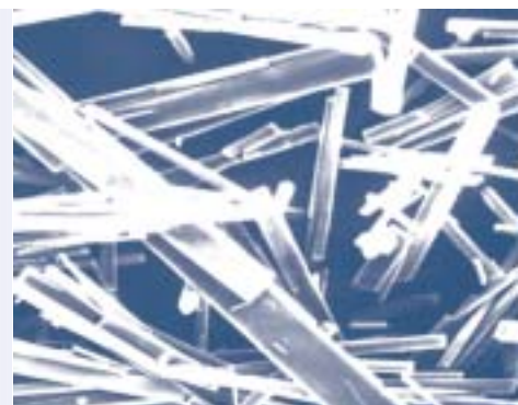
Fig. 2 The desired crystal shape as a result of controlled crystallization conditions.
