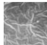
Smooth surface of an O-ring
