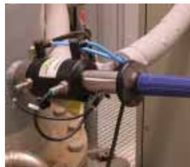
Retractable housing InTrac 777 for pH electrode InPro 3200.
