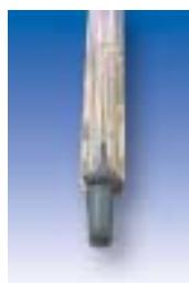
Fig.1 Dirty electrode before cleaning.
