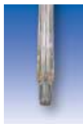
Fig.2 Electrode after cleaning.
